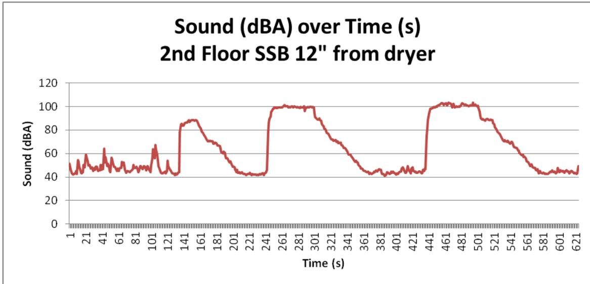
**Figure 2: Hand dryer activated and left to run, activated and hands palms down, and then activated and hands cupped, palms up. (max 103.2 dBA)**
