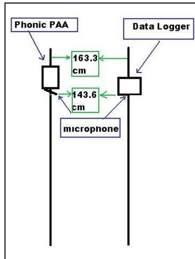
**Figure 1 - Meter stick setup with sound monitor microphones aligned to the ear canal height of 143.6 cm.**
